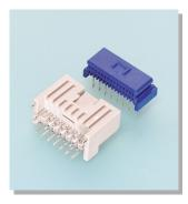
Self-supporting style board to board connectors. Both plugs and receptacles are supplied radial-tape mounted (conforming to JIS C 0805 tape specification), which can be mounted by versatile, radial component pick and place machines. Automatic mounting is possible up to 15 circuits.
