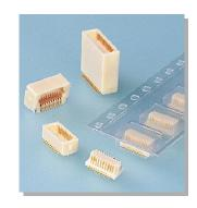
This JMC connector is 0.5 mm pitch SMT type board-to-board connector which realizes miniaturizing and space saving. Plug connector has the various connection types such as top/side entry types including the stacking height variation and receptacle connector has the fixed/absorption misalignment types.
