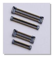
This is space saving type board-to-board connector with 0.4mm pitch, 0.8mm between PC boards and 2.0mm product width.
