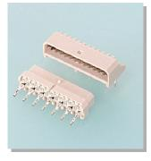
The JE connector is a compact, board-to-board connector only 6.8 mm high and 4.4 mm wide. Its mating part has a 1.25 mm pitch, single row construction. High contact pressure dual beam fork contacts are combined with a housing lock mechanism to ensure a reliable connection.
