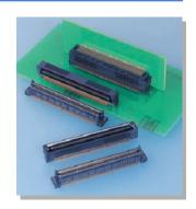
This connector is small 0.6 mm pitch dual-row board-to-board connector for high density mounting.
