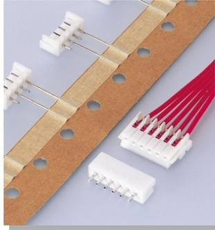
This thin type 2.5 mm pitch connector is an IDC style for PC boards. It is developed by integrating the technologies of crimp style connectors such as EH and PH, and IDC style connectors such as NR, DR, and DB. The In-line method that the wire extraction direction is perpendicular to the board provides high-density wiring.
