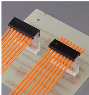
The VR series is a 3.96 mm pitch wire-to-board connector for 7 A rated power supply circuits. Furthermore, it can accommodate AWG #18 wire, which is rare for an IDC connector.
