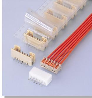
2.0 mm pitch IDC type CR connector enables to terminate with UL 1007 wire used for internal wiring of equipment specified in the Japan Electrical Appliance and Material Safety Law. This connector has a low-profile design with a mounting height of 6.9 mm and a thickness of 4.8 mm (in case of top entry type).
