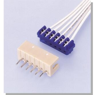
With a mounting height of 5.0 mm and a thickness of 4.8 mm (top entry type), it is the industry-leading space-saving 2.0 mm pitch mating type wire-to-board connector.
